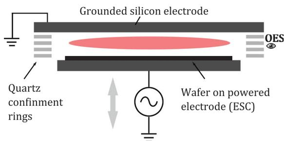
Fig. 2. (Color online) Schematic of the CCP chamber used for experimental work. Light was collected from a window on the side of the reactor. ESC, electrostatic chuck.
