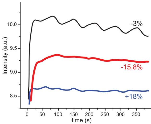
Fig. 5. (Color online) OES signals (387.6 nm) illustrating the impact of non-uniform etching (see Table I) on the interference pattern; (top line):  $-3.0\%$   $3\sigma$  uniformity (center fast); (middle line):  $-15.8\%$   $3\sigma$  uniformity (center fast), and (bottom line):  $+18\%$   $3\sigma$  uniformity (edge fast). For high enough etching nonuniformity oscillations due to interference are suppressed.
