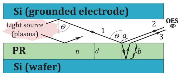
Fig. 1. (Color online) Schematic of interelectrode space (not to scale). Superposition of light beams (2) and (3) can form an interference pattern. The interference is more intense for light rays reflecting off the Si plate at the Brewster angle  $\Theta$ .
