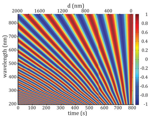
FIG. 8. (Color online) Simulation of interference pattern during etching of a 2000-nm thick photoresist film.
