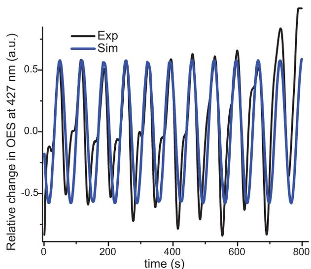
FIG. 7. (Color online) Comparison between simulation (thicker line) and experimental data (thinner line) of the interference at 427 nm during etching of a 2000-nm thick photoresist film.
