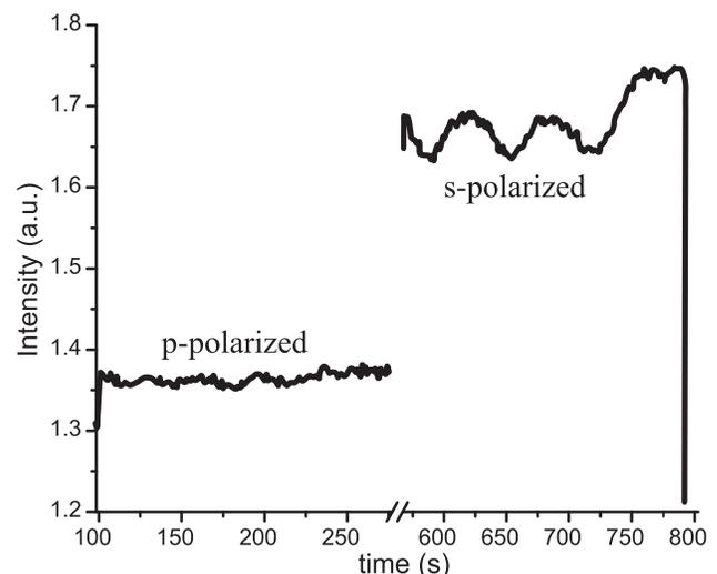
Fig. 6. OES signal for p- and s-polarized light (750 nm). Intensity oscillations are clearly visible only for the s-polarized light.
