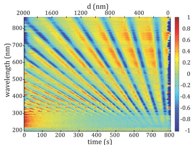
Fig. 4. (Color online) Variation of the OES intensity during etching of photoresist rescaled to the  $[-1, 1]$  interval for each wavelength. The thickness of the film, measured by ellipsometry, is shown on the upper horizontal axis.
