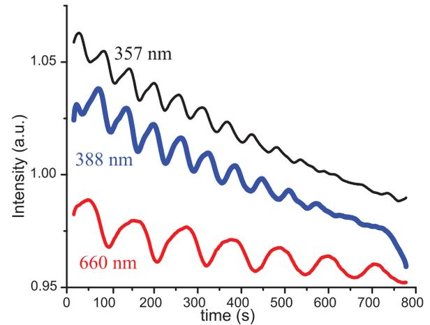
Fig. 3. (Color online) Oscillations in plasma emission during etching of photoresist. The oscillation period depends on the wavelength. The period is  $\sim 56$  s for 357 nm,  $\sim 62$  s for 388 nm, and  $\sim 110$  s for 660 nm.
