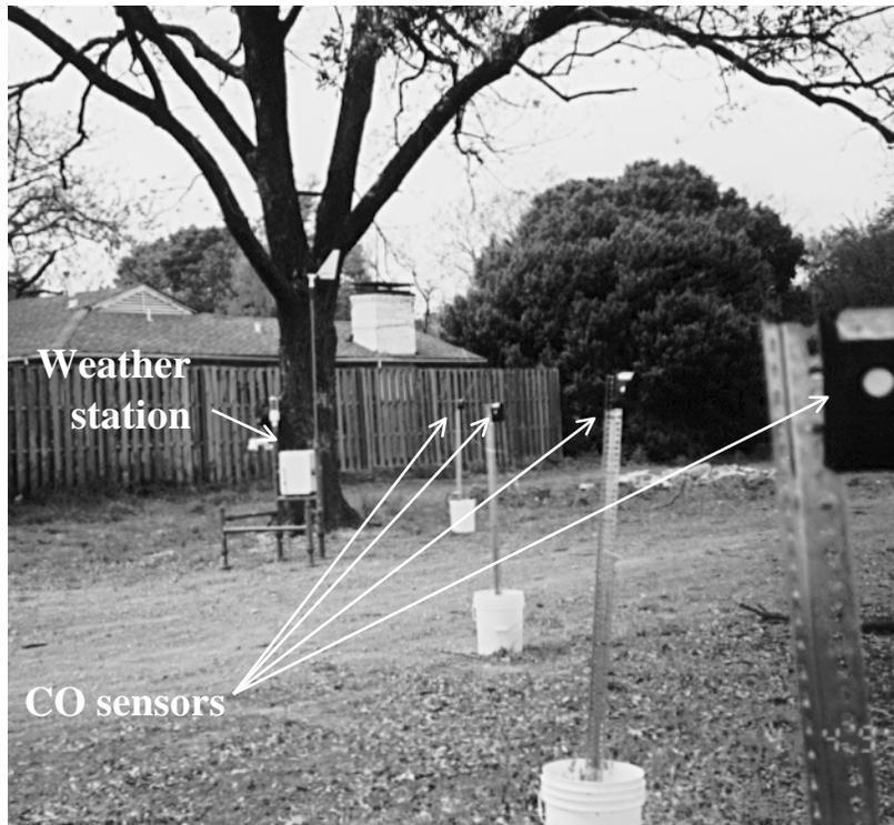
**Figure 16. Horizontally Placed CO Sensors and Weather Station for a Depressed Freeway
