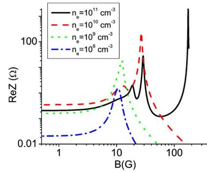
FIG. 4. (Color online). Surface resistance of warm bounded uniform Maxwellian plasmas for different electron densities as a function of the applied magnetic field. Discharge parameters: rf field frequency  $\omega/2\pi = 29 \text{ MHz}$ , electron temperature  $T_e = 4 \text{ eV}$ , electron collision frequency  $\nu = 1.2 \times 10^7 \text{ s}^{-1}$ , and the plasma half-length  $L/2 = 10.5 \text{ cm}$ .
