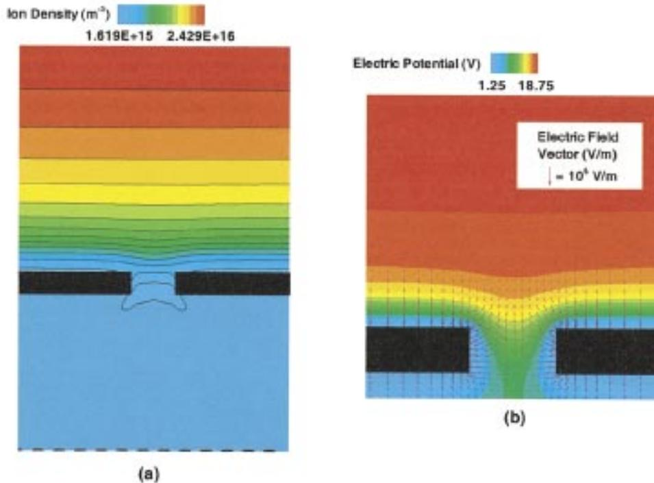
Fig. 1. Ion density (a), and potential distribution (b), near a 2-D slot. Electric field vector is also shown in Fig. 1(b). The slot width is  $508 \mu\text{m}$ . The blackened block represents the solid electrode. The dashed line at the bottom of (a) is the position where the distributions of Fig. 2 were recorded.
