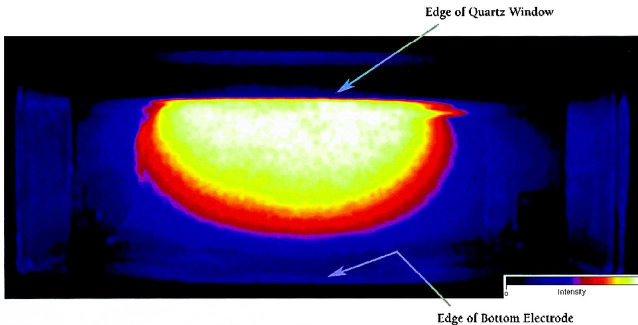
Fig. 1. Side view of a plasmoid formed at 5 mtorr. The bright structure is against the quartz window at the top and is well separated from the grounded bottom electrode. The spacing between the bottom electrode and the quartz window is 7.62 cm.
