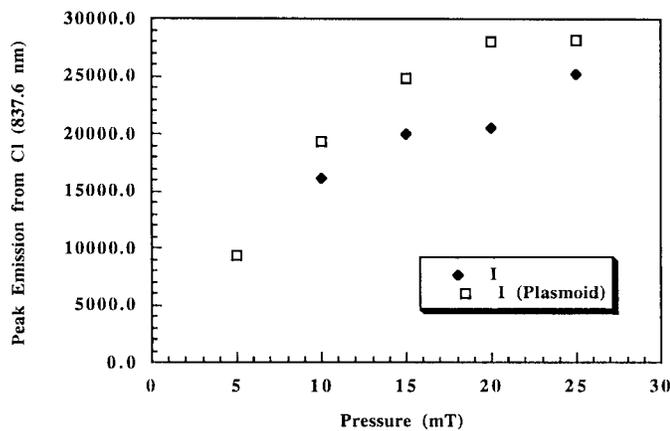
Fig. 2. Hysteresis in the Cl emission at 837.6 nm as a function of pressure in a chlorine plasma. Emission was obtained from the midplane between the quartz window and the bottom electrode and 3 cm off the reactor axis where the peak emission occurred. The filled diamonds were obtained with a conventional (diffuse) plasma, the empty squares with a plasmoid present.
