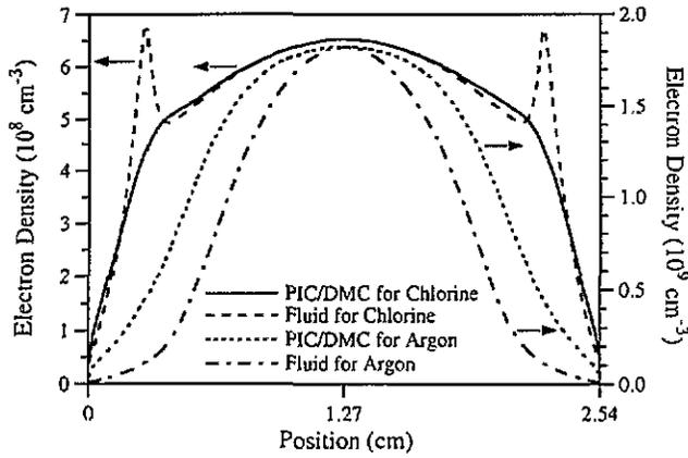
**Figure 10.** A comparison of time-average electron density as obtained by the fluid and particle-in-cell/dynamic Monte Carlo simulations.
