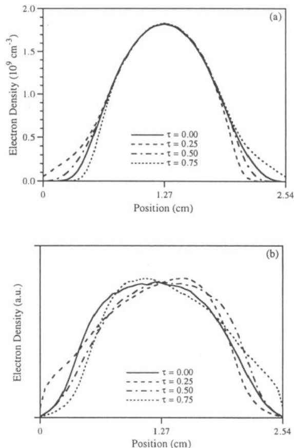
**Figure 7.** The spatiotemporal variation of the electron density in the argon discharge as obtained by (a) the fluid simulation and (b) the particle-in-cell/dynamic Monte Carlo simulation. The Monte Carlo simulation predicts only relative values of the electron density.
