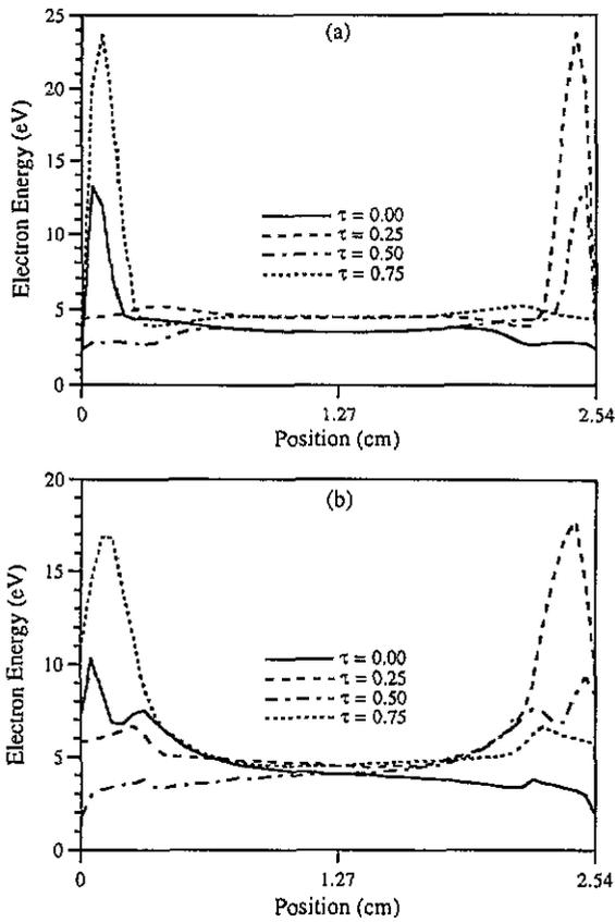
**Figure 4.** The spatiotemporal variation of electron energy in the chlorine discharge as obtained by (a) the fluid simulation and (b) the particle-in-cell/dynamic Monte Carlo simulation.
