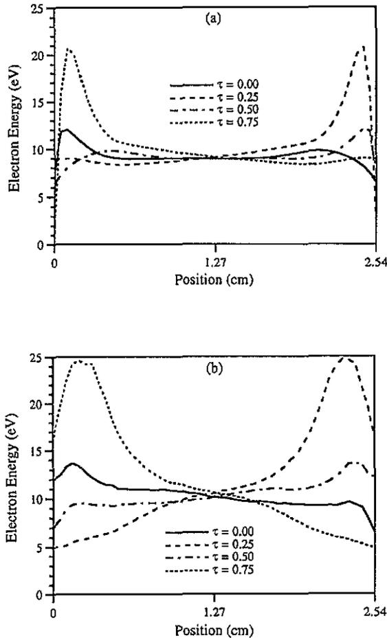
**Figure 8.** The spatiotemporal variation of electron energy in the argon discharge as obtained by (a) the fluid simulation and (b) the particle-in-cell/dynamic Monte Carlo simulation.
