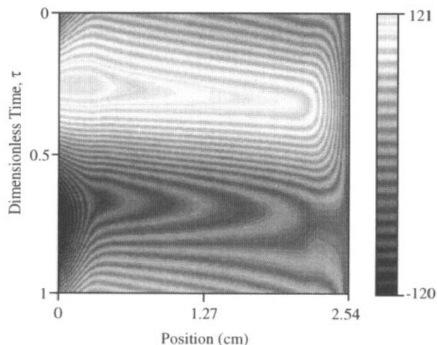
**Figure 2.** The spatiotemporal variation of potential in the chlorine discharge as obtained by the fluid simulation.
