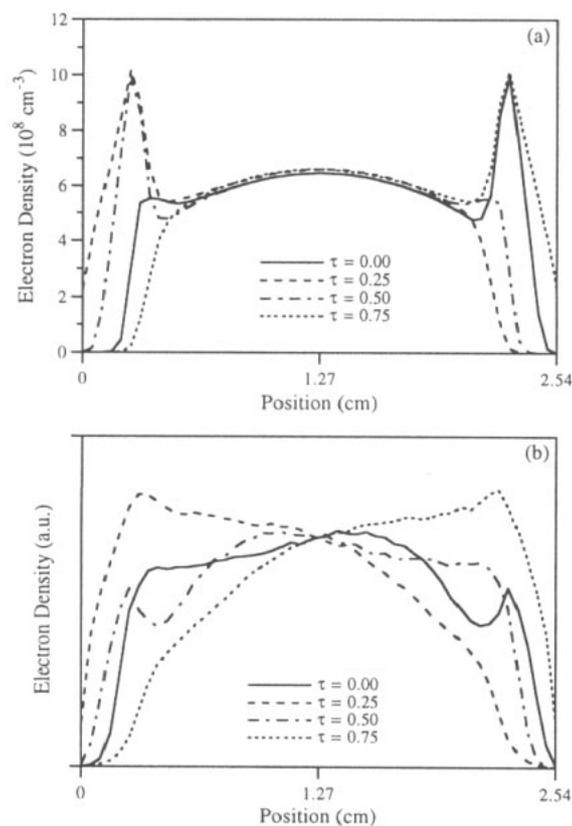
**Figure 3.** The spatiotemporal variation of the electron density in the chlorine discharge as obtained by (a) the fluid simulation and (b) the particle-in-cell/dynamic Monte Carlo simulation. The Monte Carlo simulation predicts only relative values of the electron density.
