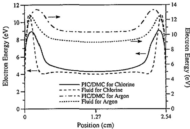
**Figure 11.** A comparison of time-average electron energy as obtained by the fluid and particle-in-cell/dynamic Monte Carlo simulations.
