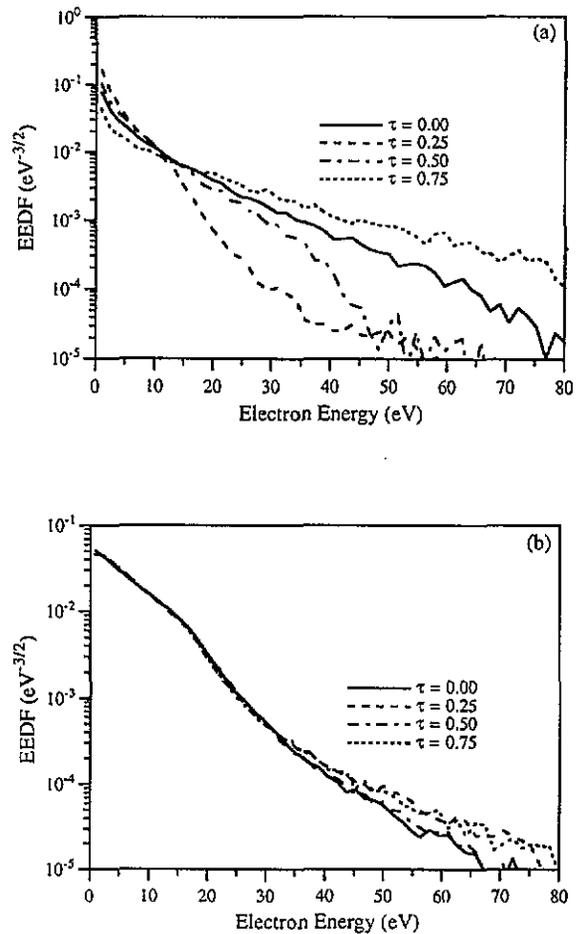
**Figure 9.** The temporal variation of the electron energy distribution function in the argon discharge at a distance of (a)  $z = 0.3$  cm and (b)  $z = 1.27$  cm from the left-hand electrode as predicted by the particle-in-cell/dynamic Monte Carlo simulation.
