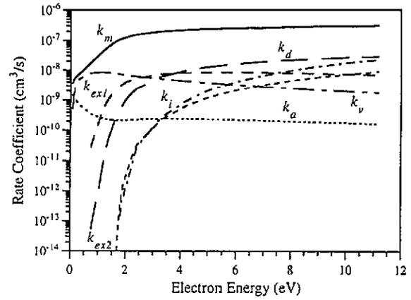
**Figure 1.** Electron-Cl<sub>2</sub> reaction rate coefficients as a function of electron energy, obtained by a zero-dimensional version of the stochastic simulation described in the text.  $k_m$ , momentum transfer;  $k_d$ , dissociative excitation to the  $C^1 \Pi$  state;  $k_{ex1}$ , excitation to the  $B^3 \Pi$  state;  $k_{ex2}$ , excitation to the  $2^1 \Pi$  and  $2^1 \Sigma$  states;  $k_i$ , ionization;  $k_v$ , vibrational excitation;  $k_a$ , attachment.
