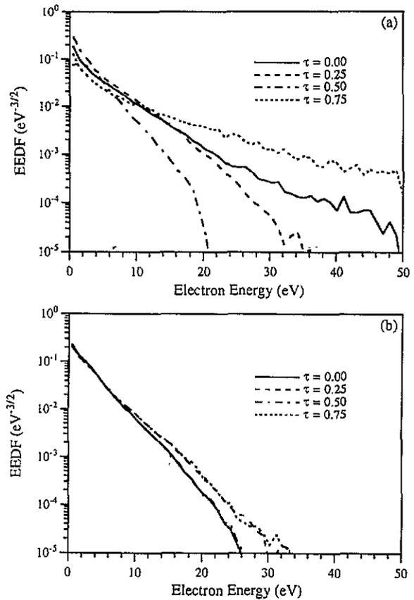
**Figure 5.** The temporal variation of the electron energy distribution function in the chlorine discharge at a distance of (a)  $z = 0.3$  cm and (b)  $z = 1.27$  cm from the left-hand electrode as predicted by the particle-in-cell/dynamic Monte Carlo simulation.
