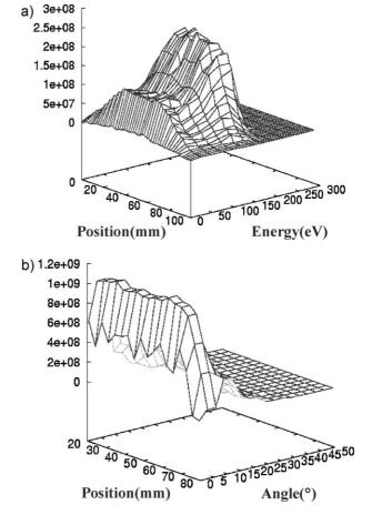
Figure 11. Fast neutral energy distribution (top) and fast neutral angular distribution (bottom) on the substrate calculated by the PIC simulation of the source shown in Figure 10, taken from  $ref.^{[13]}$
