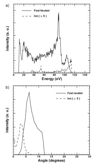
*Figure 9.* Residual ion and fast neutral energy distributions at the exit of a hole of a neutral beam source (top). Ion curve has been multiplied by 5 for clarity. Residual ion and fast neutral angular distributions at the hole exit (bottom). Ion curve has been multiplied by 5 for clarity. After ref.<sup>[53]</sup>
