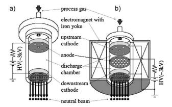
Figure 1. Neutral beam source based on volume neutralization of ions.<sup>[10]</sup> A McIlairth DC cold-cathode discharge produces ions that are extracted through holes in the (lower) cathode plate. lons are then neutralized by charge exchange with the gas downstream of the extraction electrode.
