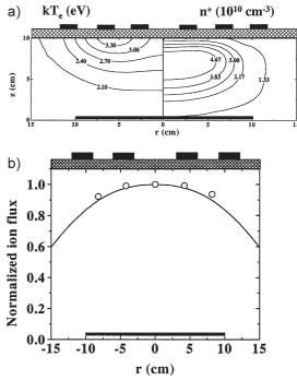
Figure 6. Electron temperature and positive ion density in a chlorine discharge<sup>[51]</sup> sustained in an inductively coupled plasma reactor at 10 mTorr and 200 W (top). Positive ion flux profile across the substrate wafer (bottom). Line is simulation prediction and points are experimental data.</sup>
