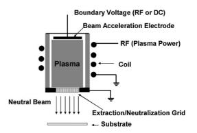
Figure 3. Neutral beam source based mainly on surface neutralization of ions.<sup>[14]</sup> lons extracted from a plasma through a grid with high aspect ratio holes are neutralized by grazing angle collisions on the internal surface of the holes of that grid.
