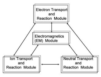
*Figure 4.* Time splitting approach in the simulation of plasma reactors. Electrons, ions and neutrals are each solved on their own time scale to speed up convergence of the simulation. The Maxwell equations (electromagnetics) are solved periodically to obtain the electric field. Information is cycled among the "modules" until a steady state is reached.<sup>[29]</sup>
