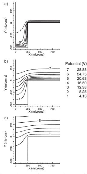
Figure 7. Electric potential contours around a 500  $\mu$ m-wide and 500  $\mu$ m-deep trench at  $\tau_{rf} = 0$ : a)  $L_{sh} = 108 \ \mu$ m ( $L_{sh}/D = 0.22$ ); b)  $L_{sh} = 468 \ \mu$ m ( $L_{sh}/D = 0.94$ ); c)  $L_{sh} = 1281 \ \mu$ m ( $L_{sh}/D = 2.6$ ).  $L_{sh}$  is the time-average sheath thickness calculated far away from the trench, where the sheath was one-dimensional.<sup>[46]</sup>
