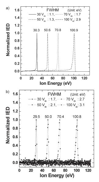
*Figure 12.* Nearly monoenergetic distribution of extracted ions for different DC bias potentials (30, 50, 70, and 100 V) applied in the afterglow (RF power off, top).<sup>[48]</sup> Experimental data from ref.<sup>[56]</sup> for the same conditions as in the simulation (bottom, FWHM = full width at half maximum).
