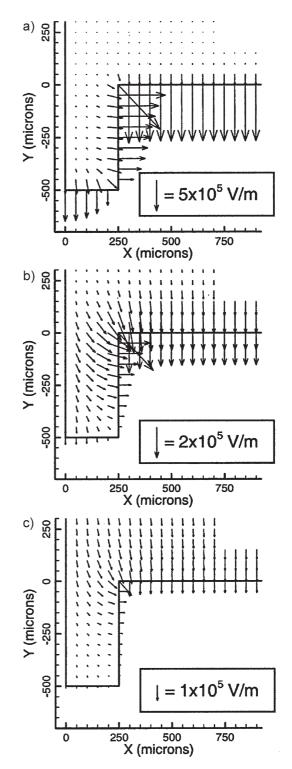
Figure 8. Electric field vector plots for the conditions of Figure 7: a)  $L_{sh} = 108 \ \mu m \ (L_{sh}/D = 0.22);$  b)  $L_{sh} = 468 \ \mu m \ (L_{sh}/D = 0.94);$ c)  $L_{sh} = 1281 \ \mu m \ (L_{sh}/D = 2.6).^{[46]}$
