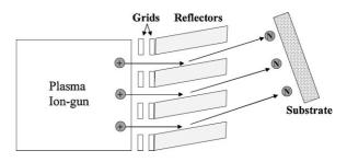
Figure 2. Neutral beam source based on surface neutralization of ions.<sup>[13]</sup> lons extracted from a gridded ion beam source are neutralized by grazing angle collisions on reflector plates.
