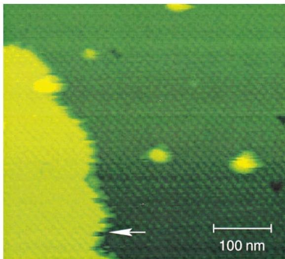
**Figure 5.** Surface scan immediately after Figure 4, arrow indicates location of monitoring in Figure 4. Clusters and vacancies similar to those in Figure 1 seen on lower terrace.
