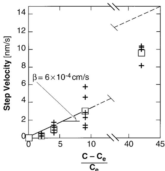
**Figure 6.** Step velocities  $v$  determined by comparing step positions within 44–47 seconds, plotted as function of concentration supersaturation  $(C - C_e) \cdot C_e^{-1}$ . +, individual determinations; data scatter reflects the stochastic nature of crystal growth at the molecular level; □, average  $v$  for each concentration. Continuous line corresponds to shown step kinetic coefficient  $\beta$ .
