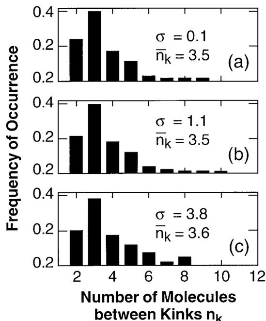
**Figure 2.** Distribution of number of molecules between kinks on steps located  $>0.5 \mu\text{m}$  apart, obtained from images similar to Figure 1 at the three supersaturations  $\sigma$  indicated in the plots, the mean values of the distributions for each case are also shown. The protein concentrations corresponding to these  $\sigma$ 's are (a)  $25 \mu\text{g/ml}$ , (b)  $70 \mu\text{g/ml}$  and (c)  $1 \text{ mg/ml}$ .
