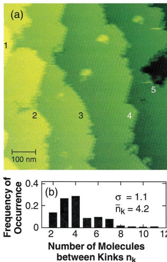
**Figure 3.** (a) Structure of steps and (b) kink distribution for closely spaced steps at apoferritin concentration of  $70 \mu\text{g/ml}$ , supersaturation  $\sigma = 1.1$ . Clusters similar to the one in Figure 1 are seen on the terraces behind steps 3, 4, and 5 in (a).
