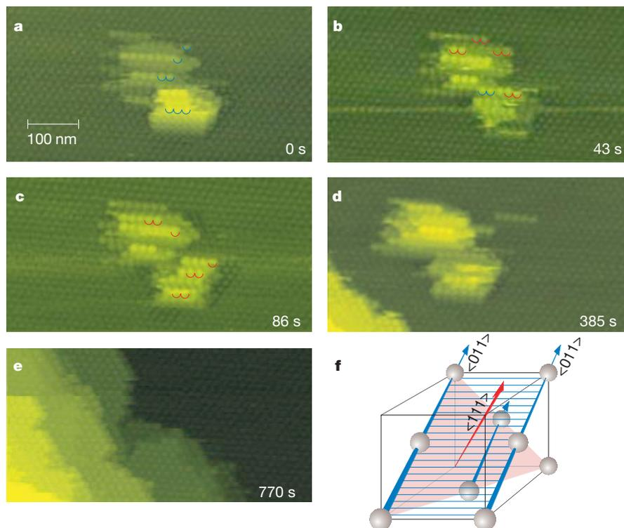
**Figure 1** Near-critical-size cluster on the (111) face of an apoferritin crystal at supersaturation  $\sigma = 1.1$ . **a–c**, Molecules attach and detach from the cluster. Molecules that are missing in the next frame are highlighted in blue, those that have appeared after the previous frame were captured are highlighted in red. **d, e**, An advancing step pushes the cluster back into the solution. The step velocity is  $0.6 \text{ nm s}^{-1}$ , close to the fastest step
