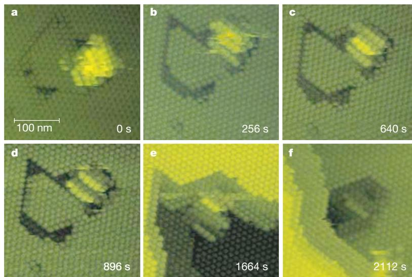
**Figure 2** A slowly dissolving cluster at  $\sigma = 1.6$ . **a–d**, The top layer of the cluster is gradually disappearing because more molecules detach than attach to the cluster. The fraction of the top crystal layer originating from the cluster is out of registry with the remaining part. **e, f**, A few steps belonging to the crystal surround the cluster. Note the
