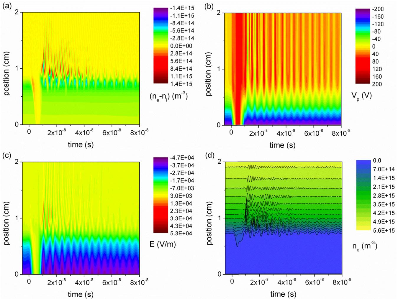
Fig. 1. Spatiotemporal profile of plasma characteristics at the powered electrode sheath of a CCP driven by asymmetric trapezoidal voltage pulses for times around the onset of the instability. (a) Net charge density ( $n_e - n_i$ ). (b) Electric potential. (c) Electric field. (d) Electron number density.
