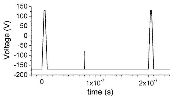
Fig. 2. Applied voltage waveform with a frequency of 5 MHz. The time window shown in Fig. 1 starts at  $t = 0$  and ends at the time indicated by the vertical arrow.
