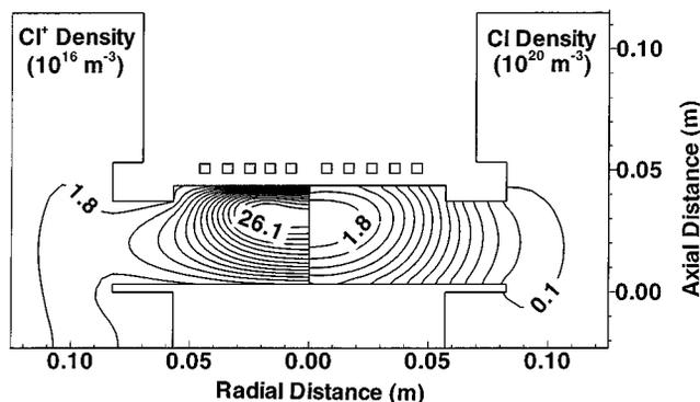
FIG. 1.  $\text{Cl}^+$  ion (left-hand side) and Cl atom (right-hand side) number density distributions for 20 sccm, 180 W, 20 mTorr chlorine plasma sustained by an inductively coupled source in a Gaseous Electronics Conference cell geometry. A cross section of the planar coil is also shown.
