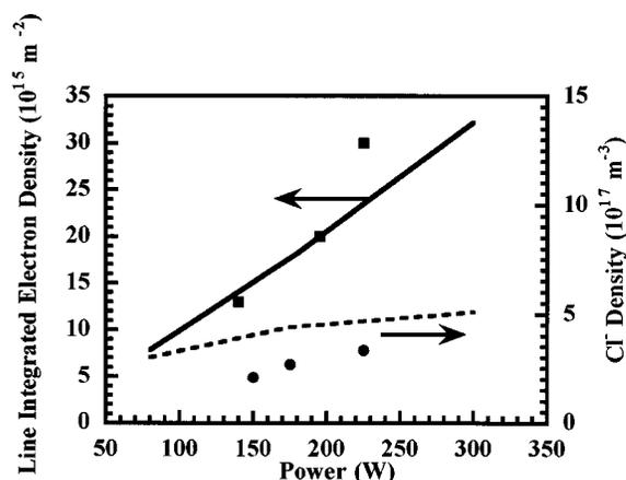
FIG. 2. Comparison between simulation results (lines) and experimental data (points) for a 20 mTorr chlorine plasma. Left-hand side axis: line-integrated electron density through the reactor midplane; solid squares are data from Ref. 15. Right-hand side axis: negative ion density at the reactor center; solid circles are data from Ref. 18.
