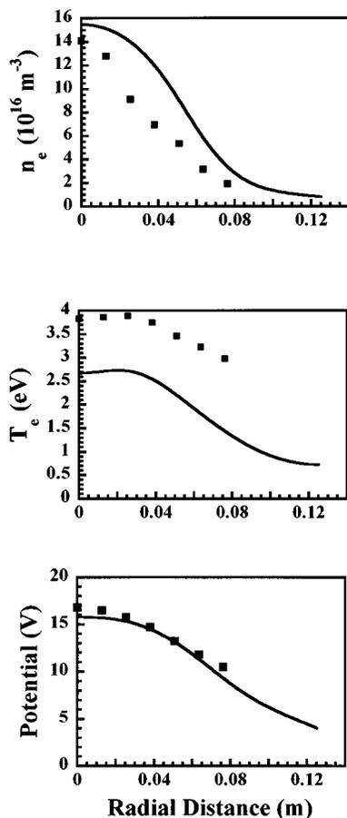
FIG. 3. Comparison between simulation results (lines) and experimental data (points, Refs. 15 and 18) of spatially resolved electron density (top), electron temperature (middle), and plasma potential (bottom) in a chlorine plasma. Conditions: 180 W and 20 mTorr.
